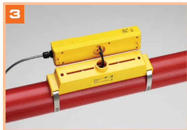
Connect power and sensors to electronic assembly
